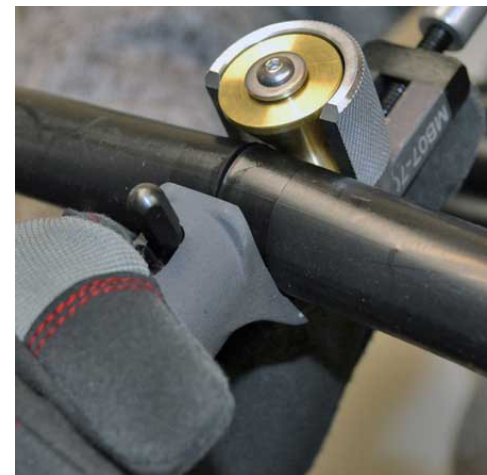
Ergonomic handle provides additional leverage for ring cutting operations
