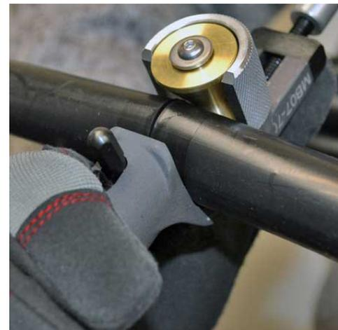
*Ergonomic handle provides additional leverage for ring cutting operations*
